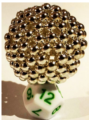
Figure 2. A dipole cluster from 5 mm neodymium spheres with dodecahedral symmetry. The magnetic order of the dipole orientation will in general reduce that symmetry to a subgroup, which can be interactively explored [1].
