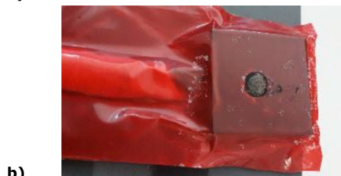
Fig. 1) a) Electrochemical setup and b) loaded sample holder for IONP
