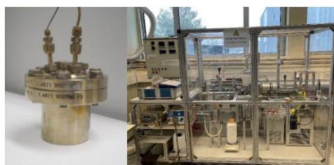
Fig. 2. Batch autoclave and plant for continuous hydrothermal synthesis in \text{scH}_2\text{O} .
