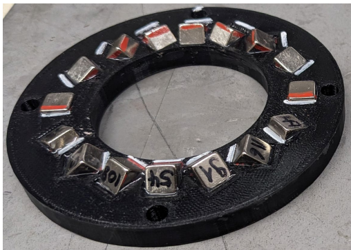
Figure 1. Sixteen neodymium 1 cm 3 cubes form a prototype used for the focussed configuration measurements in [4].
