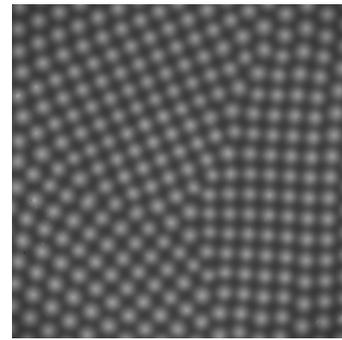
Figure 3: Radioscopic image of the Rosensweig peaks in our ferrogel (19\*19cm).
