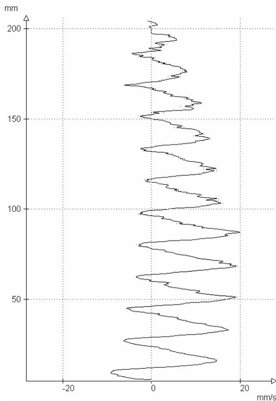
**Fig. 2a:** Snapshot 1 of a wavy vortex flow (WVF) at  $Re=160$  for the inner cylinder and  $Re=45$  for the counter rotating outer cylinder.
