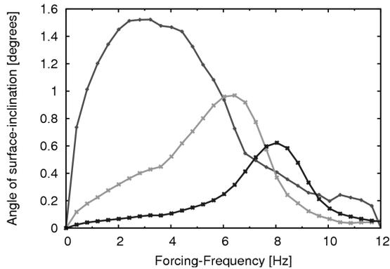
Figure 3: Angle of surface inclination as a function of driving frequency for different magnetic inductions
