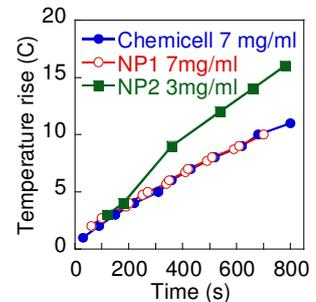
**Figure 3:** Magnetic heating of magnetite/maghemite nanoparticles in a 140 Oe field at 138 kHz.
