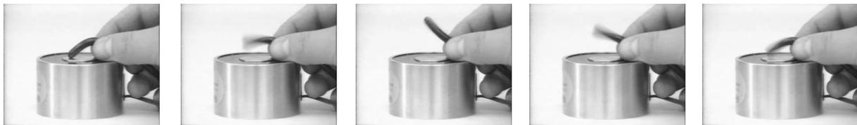
Fig. 1 Snapshot of shape change of a magnetite-loaded PDMS gel due to modulated magnetic field. The frequency of the field is 40 Hz.
