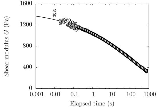
Figure 4: The force response to a jump in the deformation. The solid line displays a fit to Eq. (2) with the parameters  $G_{theo} = 1480$  Pa,  $t_0 = 127$  s and  $\beta = 0.218$ .
