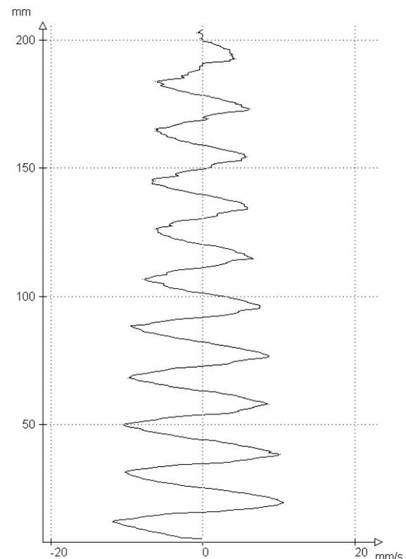
**Fig. 1:** Axial sinusoidal velocity profile for  $Re=118$  for the inner cylinder,  $Re=0$  for the outer cylinder and the US-transducer being placed at the outer cylinder wall.
