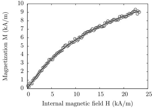
Figure 3: Magnetization curve of the ball.
