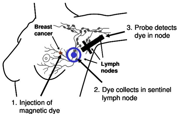
**Figure 1:** An intra-operative medical device for breast cancer surgery which uses a high-sensitivity, high- $T_c$  SQUID based probe.
