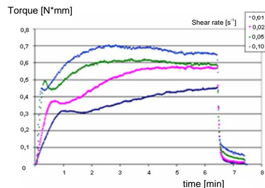
Figure 1. A long-time reaction of rheometers torque sensor to the shear stress stepwise change [5].
