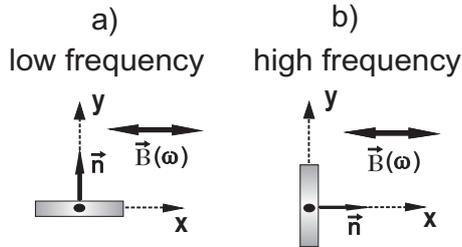
Figure 1: The two different orientations of the pendulum for low and high driving frequencies.
