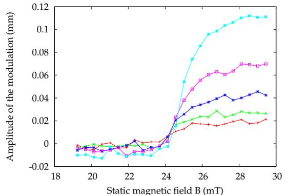
Figure 2: Amplitude of the modulation of the surface deflection in response to a modulated magnetic field
