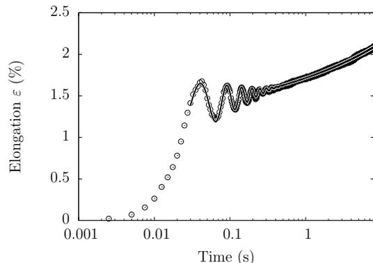
Figure 2: Elastic response of the ball, when a magnetic field is suddenly applied. The solid line represents a fit with a harmonic oscillator.
