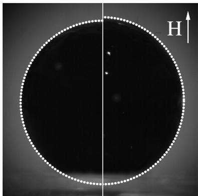
Figure 1: Image of the symmetrical (left) and distorted ball (right). The dotted line displays a fit with a circle (left) and an ellipse (right).
