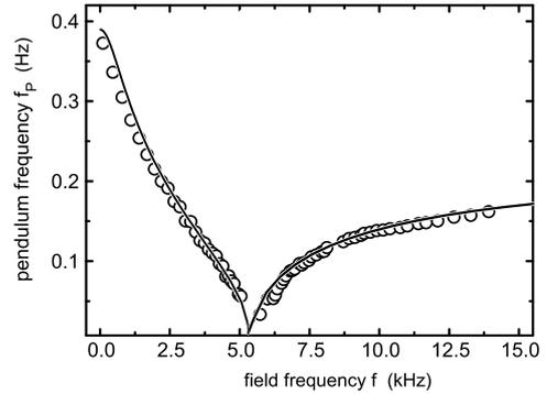
Figure 2: Pendulum frequency versus driving frequency for a constant driving amplitude. The flip occurs for  $f_P = 0$  at  $f \approx 5.2$  kHz. From [4].
