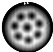
Figure 1: Radioscopic image of the Rosensweig peaks in our ferrogel.
