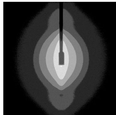
*Scattering pattern with external magnetic field ( $B_0 = 0.1 T$ ) perpendicular to the primary beam.*
