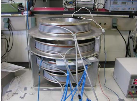
fig. 1: Fanselau arrangement to generate a magnetic field strength up to 25 kA/m
