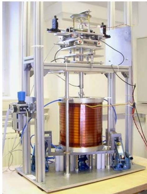
fig. 1: The shear stress controlled rheometer for the investigations of the yield stress in ferrofluids.
